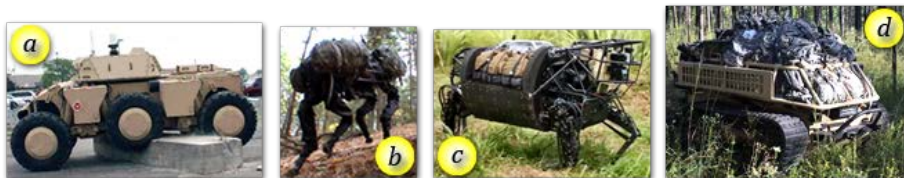
Figure 5: Example UGVs for military logistic support, (a) APD, (b) Big Dog, (c) LS3 Cujo, and (d) RS2-H1 SMET ( Army Guide, 2020a; DefPost, 2020; Hua, 2020 )
