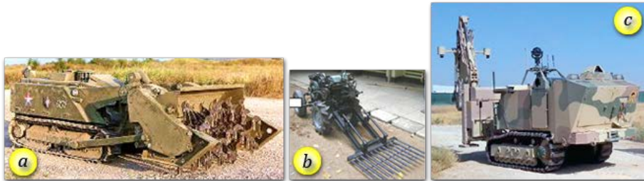
Figure 3: Some autonomous vehicles (UGVs) used for field minesweeping, (a) URAN-6, (b) RAMS, and (c) Rout Clearing System (detection unit) (Hemapala, & Razzoli, 2012; Dilipraj, 2016; Smolarek, 2019)
