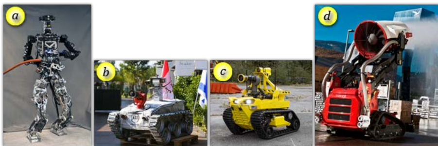
Figure 8: Fire-fighting UGVs, (a) SAFFiR, (b) FFR-1, (c) Thermite, and (d) TAF-20 (Tan et al., 2013; AlHaza et al., 2015; Kim, & Lattimer, 2015; Nuță et al., 2015; Liu, 2016; AirCore TAF35, 2020)
