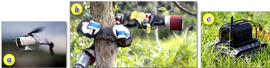
Figure 4: Some examples of autonomous robots for military surveillance and reconnaissance, (a) PD-100, (b) Modular snake robot, and (c) RABE ( Wright et al., 2012; Smolarek, 2019; Abiodun, & Taofeek, 2020 )
