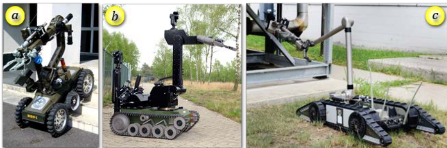
Figure 7: Example of some military robots used for Bomb disposal and Chemical detection, (a) DAKSH, (b) tEODor, and (c) PackBot 510 ( Antal, 2016; Dilipraj, 2016; Smolarek, 2019 )
