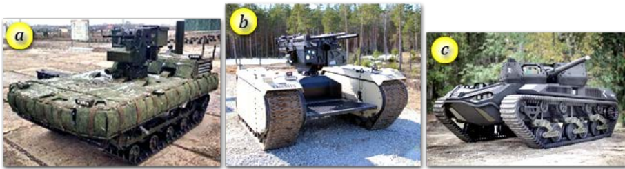
Figure 9: Armed UGVs, (a) WOLF-2, (b) THeMIS, and (c) Ripsaw M5 RCV (Dilipraj, 2016; Mizokami, 2019; Army Technology, 2020)
